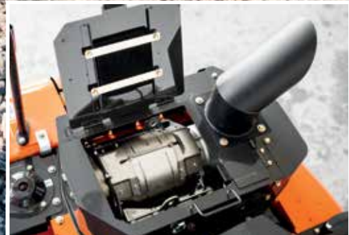
The SCR system reduces emissions and noise levels.
